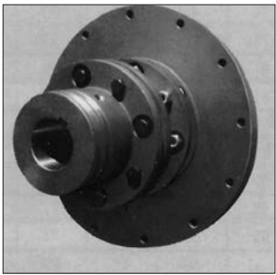
Coupling for fly-wheels: Features construction capable of withstanding the reversal and vibration torques of engine drives and reciprocal compressors.
